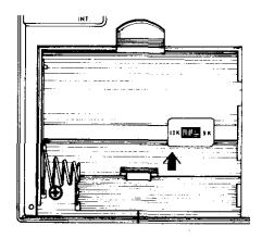
Insert six D batteries in the main battery compartment. Position them as shown in the illustration on the back of the radio. For best results, use alkaline batteries such as Radio Shack® Cat. No. 23-550.
